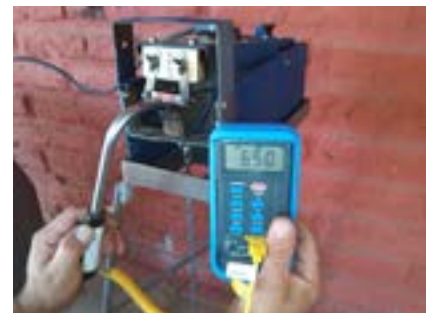
Pyrometer indicating proper blade temperature of 650°C.
